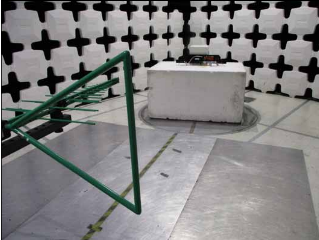
Test Setup for Radiated Emissions: Below 1GHz, Horizontal Polarization
