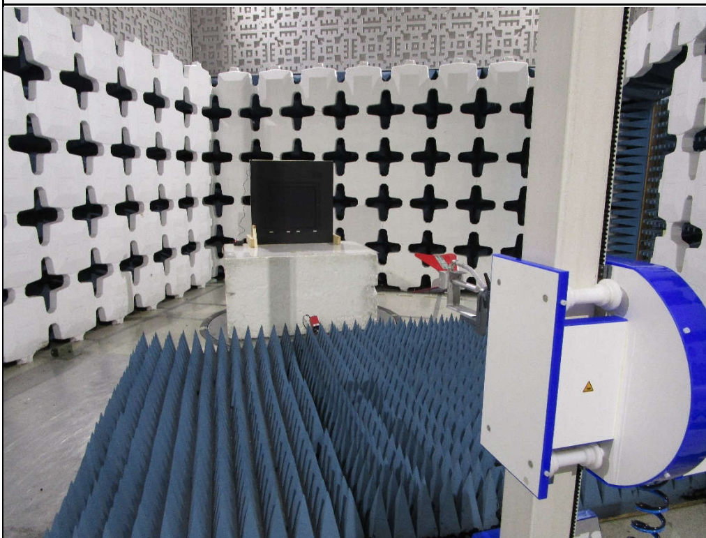
Test Setup for Spurious Radiated Emissions, 1 – 18GHz – Antenna Polarization Vertical
