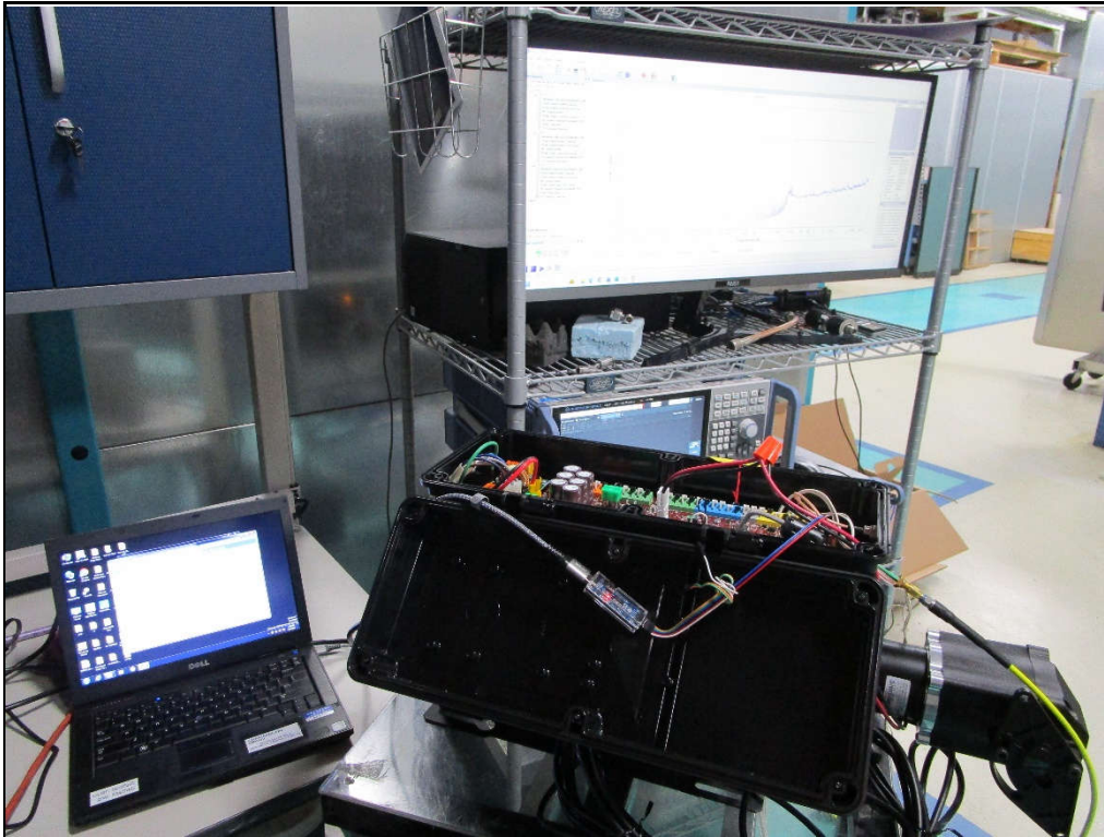
Test Setup for Antenna Conducted Tests
