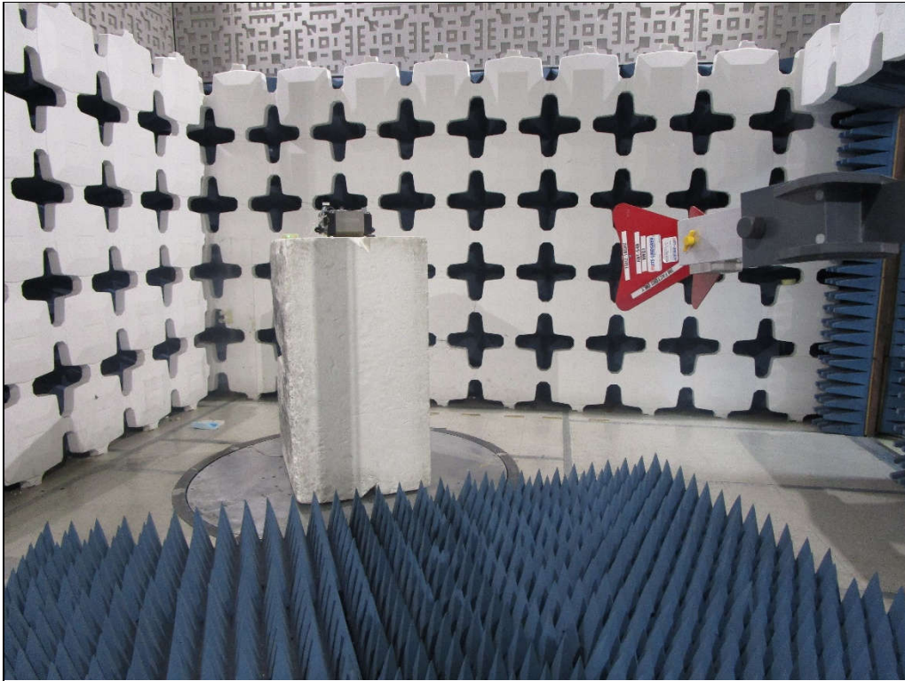
Test Setup for Spurious Emissions: Above 1GHz, Horizontal Polarization
