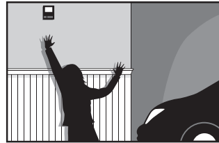
The wall-mounted push button should be out of reach of children, at least 5 feet from the nearest standing surface and away from all moving parts. Mount and use the button where you can clearly see the closing garage door.
