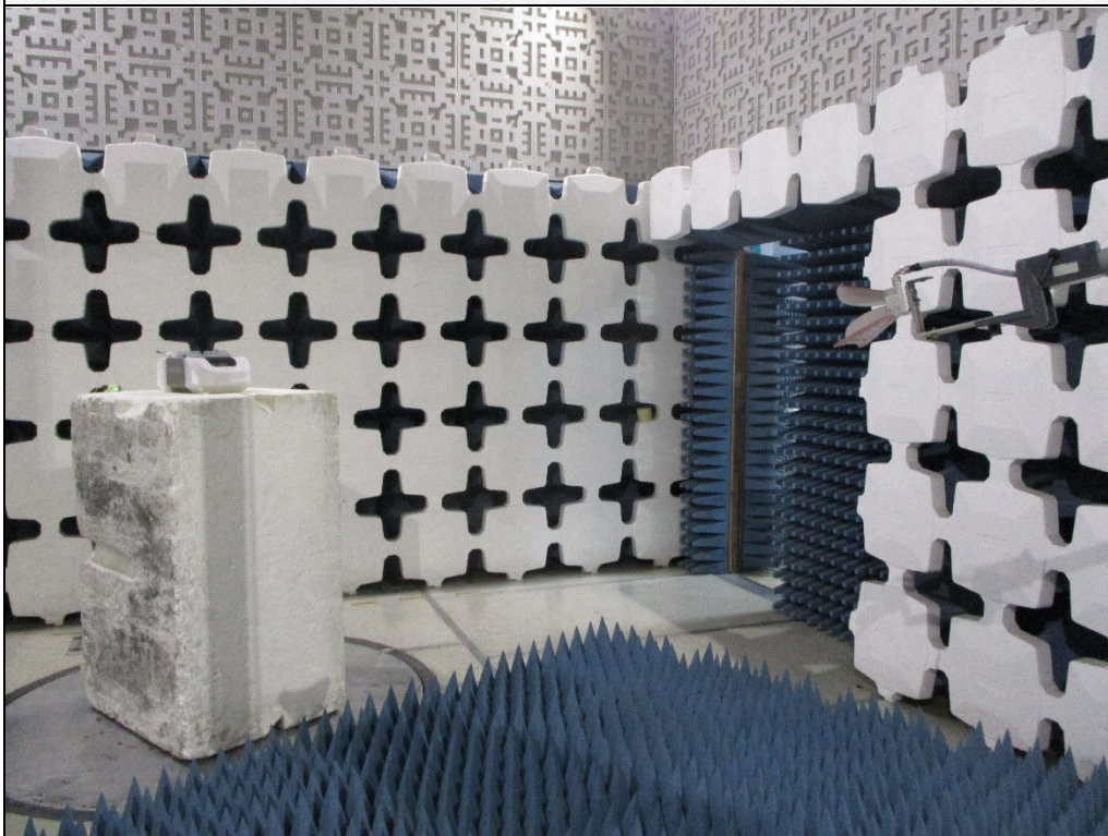
Test Setup for Spurious Radiated Emissions, 1 – 10GHz – Antenna Polarization Vertical
