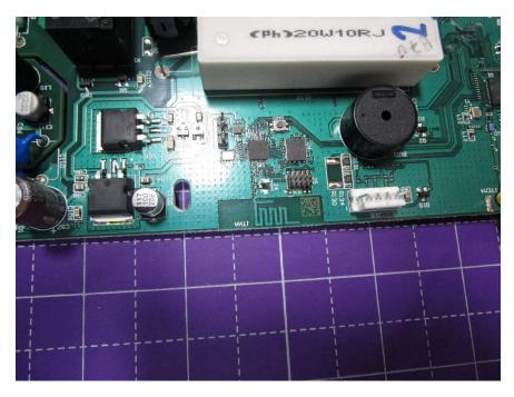
7.2 mm 20 AWG monopole wire antenna for the FHSS transmitter
