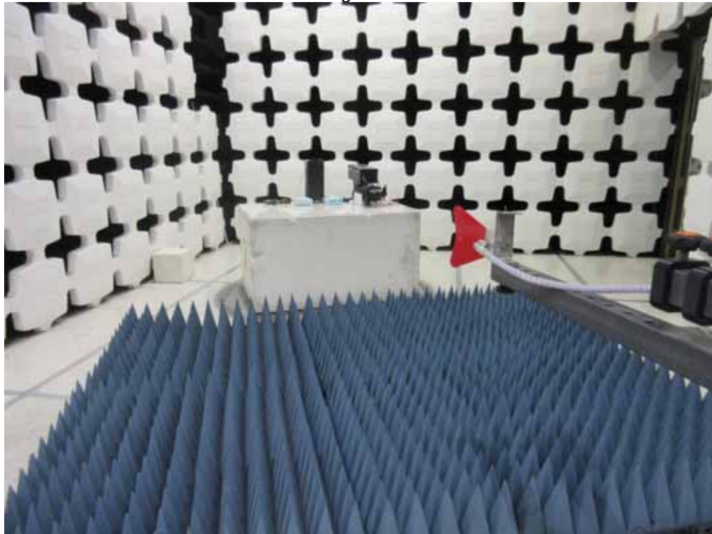
Test Setup for Radiated Emissions (Receiver) – 1 to 10GHz, Horizontal Polarization
