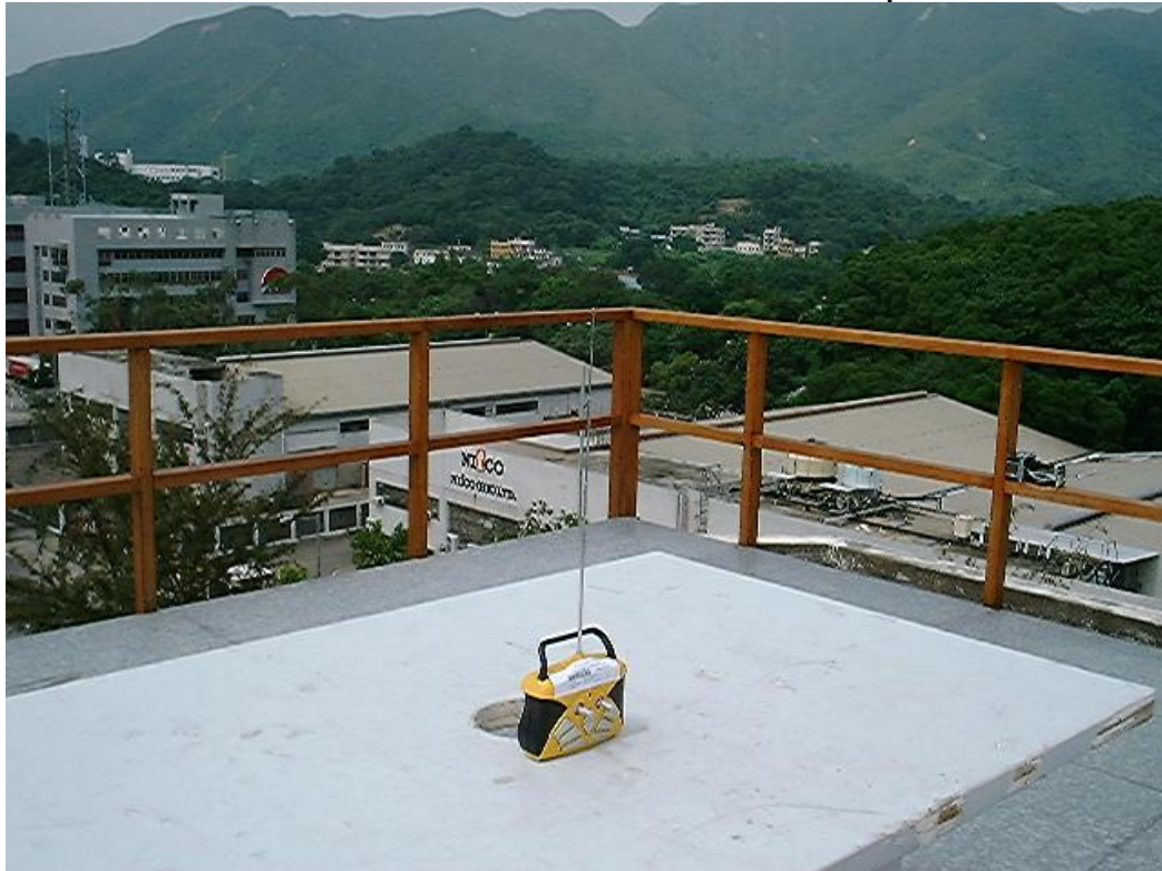
Measurement of Radiated Emission Test Set Up
