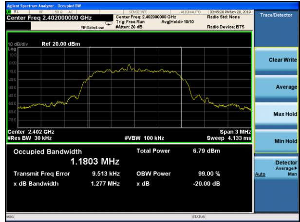
20dB Bandwidth plot on channel 39 (2Mbps)
