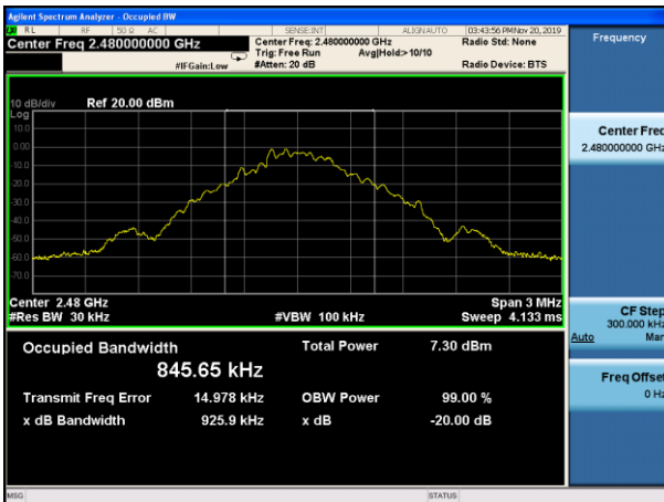
20dB Bandwidth plot on channel 78 (1Mbps)
