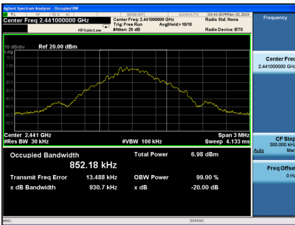
20dB Bandwidth plot on channel 39 (1Mbps)
