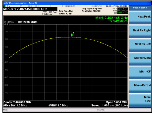
Peak output Power plot on channel 39 (2Mbps)
