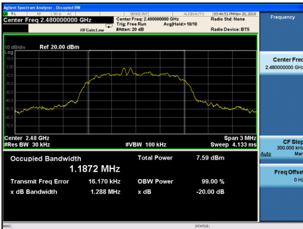
20dB Bandwidth plot on channel 78 (3Mbps)
