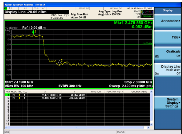
8-DPSK: Band Edge-High Channel (Hopping Mode)
