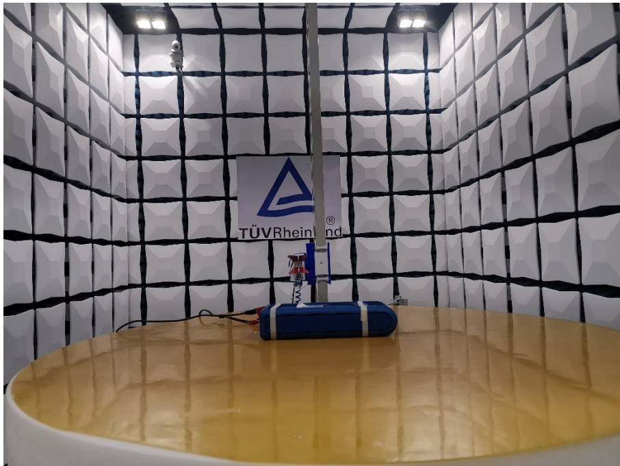
Photograph 2: Set-up for Radiated Spurious Emission, Above 1GHz
