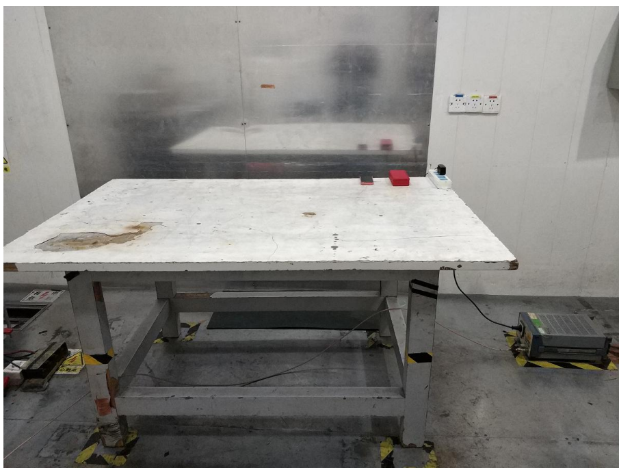
Photograph 3: Set-up for Conducted Emission on AC Mains
