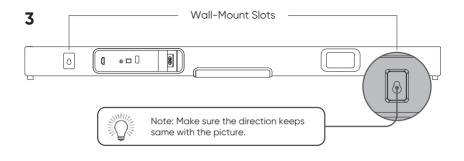
Hang the Soundbar on the wall mount screws then slide down to lock in place.
