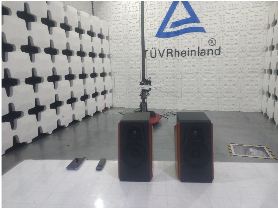
Photograph 4: Set-up for Radiated Emission, below 1GHz
