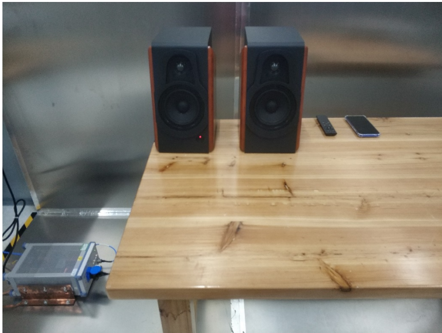
Photograph 3: Set-up for Conducted Emission on AC Mains
