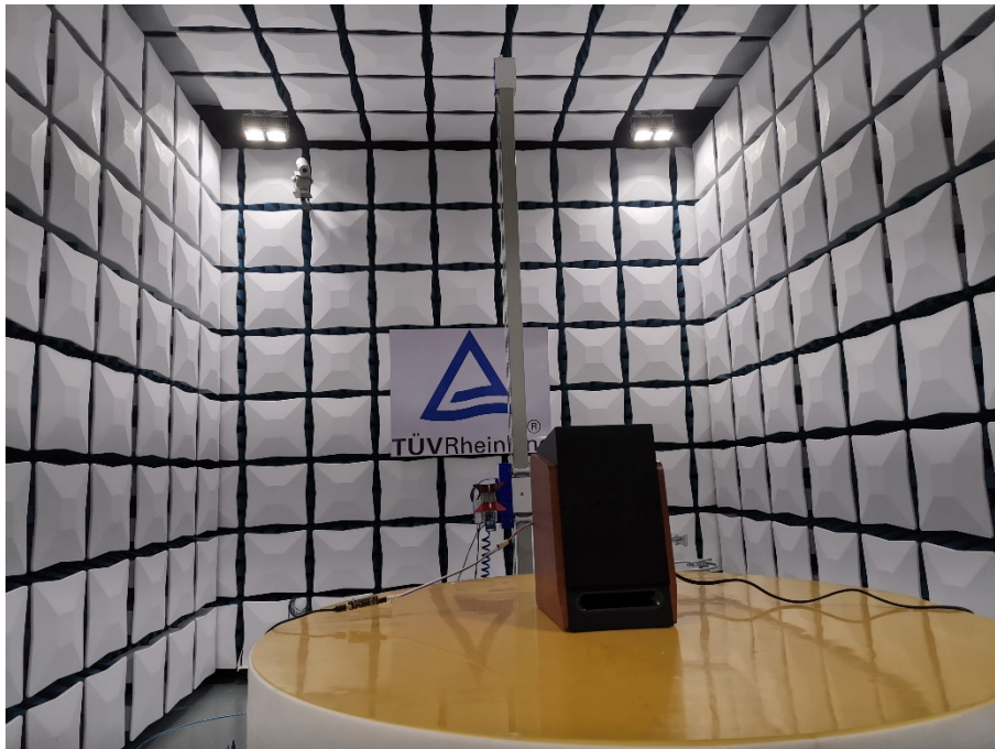
Photograph 2: Set-up for Radiated Spurious Emission, Above 1GHz
