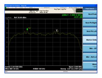
(3Mbps) Channel Separation plot on channel 77-78
