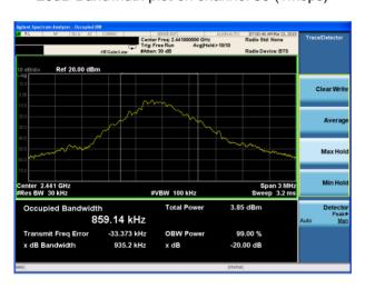
20dB Bandwidth plot on channel 39 (2Mbps)
