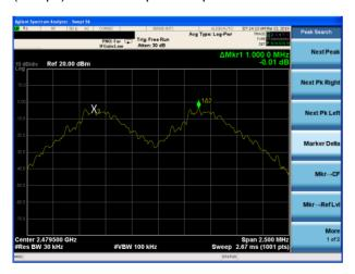
(2Mbps) Channel Separation plot on channel 77-78
