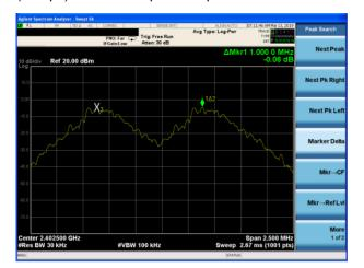
(2Mbps) Channel Separation plot on channel 00-01
