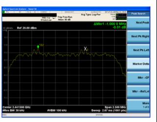
(1Mbps) Channel Separation plot on channel 77-78
