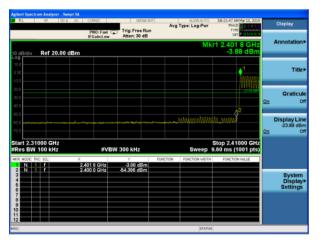
GFSK: Band Edge-High Channel (Hopping Mode)
