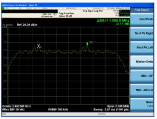
(1Mbps) Channel Separation plot on channel 39-40
