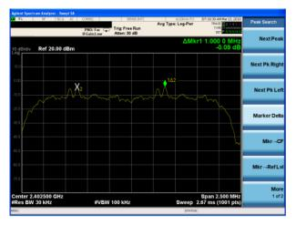
(3Mbps) Channel Separation plot on channel 39-40
