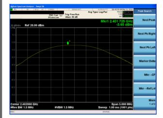
Peak output Power plot on channel 00 (2Mbps)
