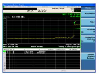
8-DPSK: Band Edge-High Channel (Hopping Mode)
