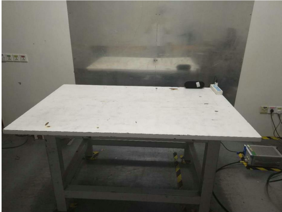
Photograph 1: Set-up for Conducted Emission on AC Mains
