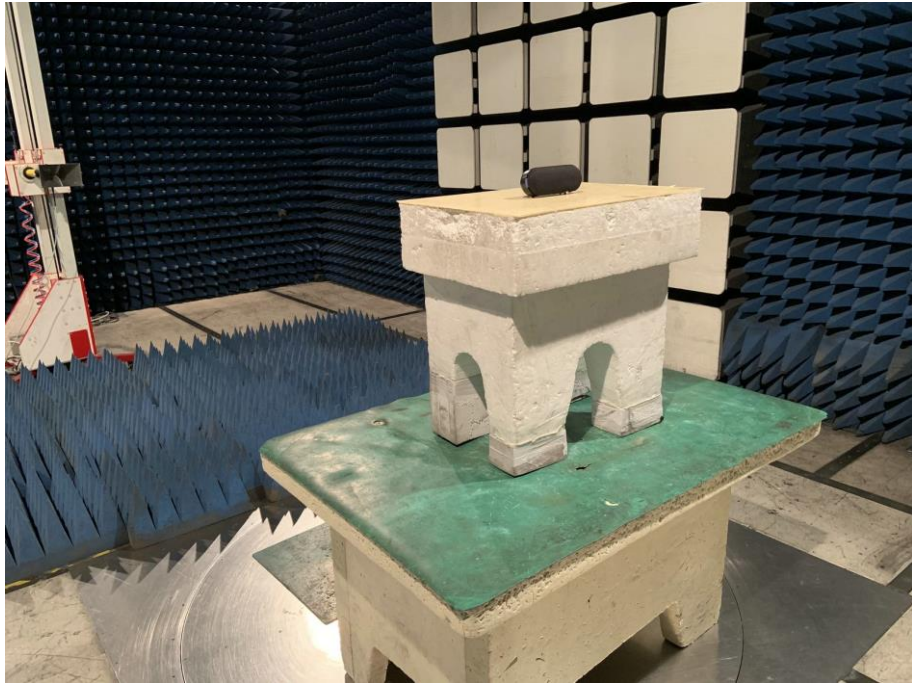
Photograph 3: Set-up for Radiated Spurious Emission, 1GHz - 18GHz
