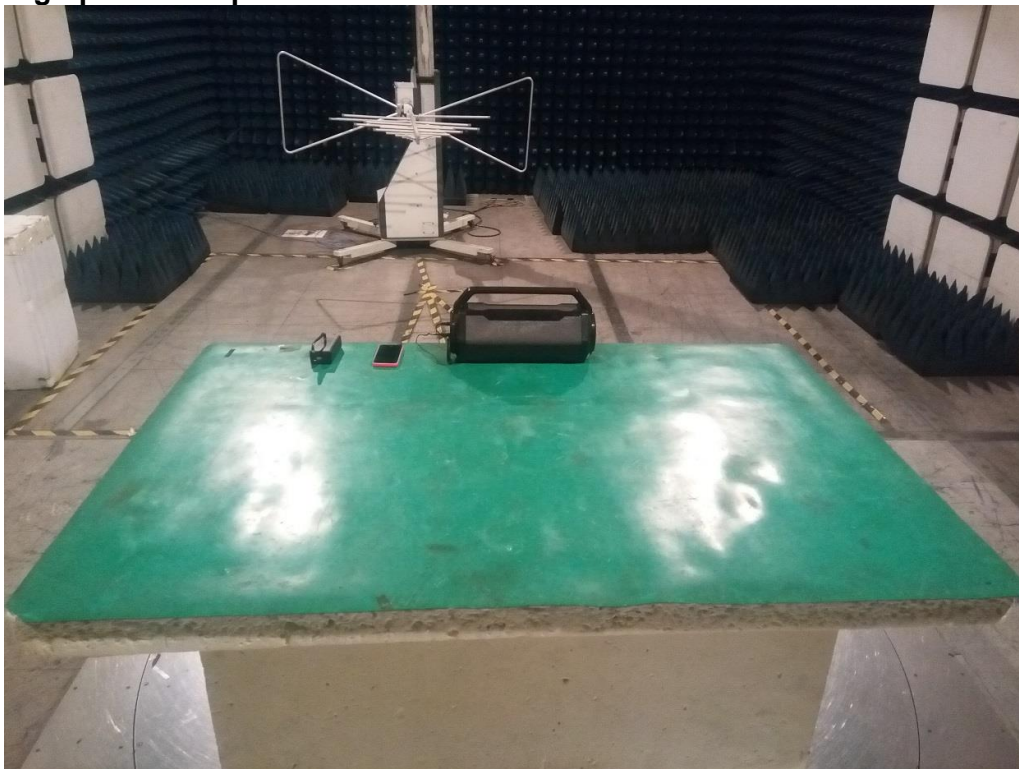
Photograph 4: Set-up for Radiated Emissions
