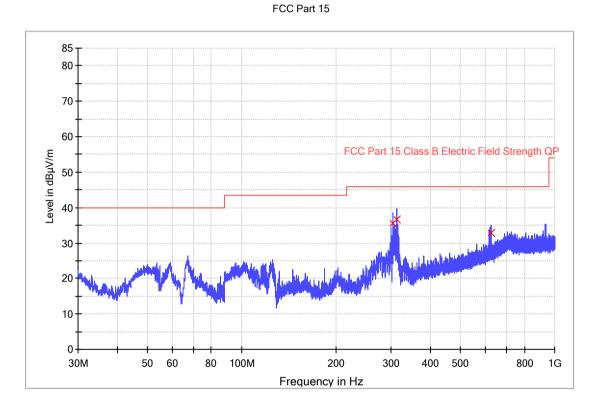
Meas. Margin -Limit – Quasi Peak Bandwidth Height Frequency Corr. Polarization QPK Time **QPK** (MHz) (dBµV/m) (kHz) (dB/m) (cm) (ms) (dB) (dBµV/m) 35.6 120.000 20.5 303.831000 1000.0 100.0 v 10.4 46.0 311.979000 36.7 1000.0 120.000 100.0 20.9 9.3 46.0 v 628.134333 33.0 1000.0 120.000 100.0 29.5 13.0 46.0 v
