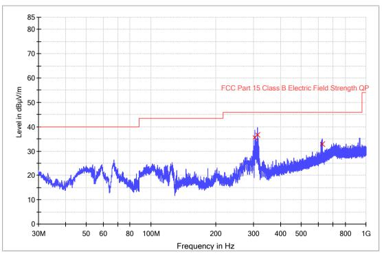
Meas. Margin -Limit – Quasi Peak Bandwidth Height Frequency Corr. Polarization QPK Time **QPK** (MHz) (dBµV/m) (kHz) (dB/m) (cm) (ms) (dB) (dBµV/m) 303.831000 35.6 120.000 20.5 1000.0 100.0 v 10.4 46.0 311.979000 36.7 1000.0 120.000 100.0 20.9 9.3 46.0 v 628.134333 33.0 1000.0 120.000 100.0 29.5 13.0 46.0 v
