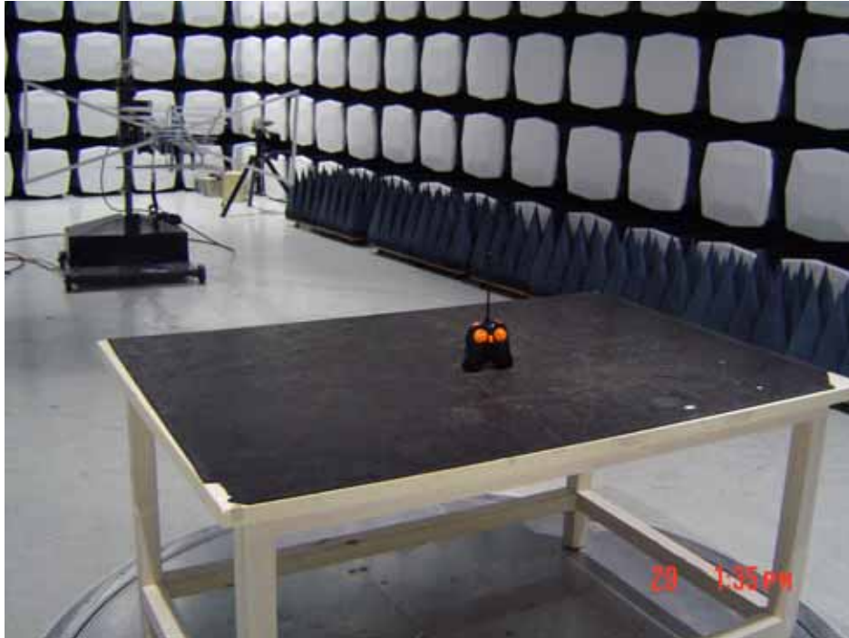
Radiation Emission Test setup
