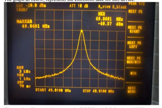
The results: The unit does meet the FCC Part 15 C Section 15.235 requirements.
