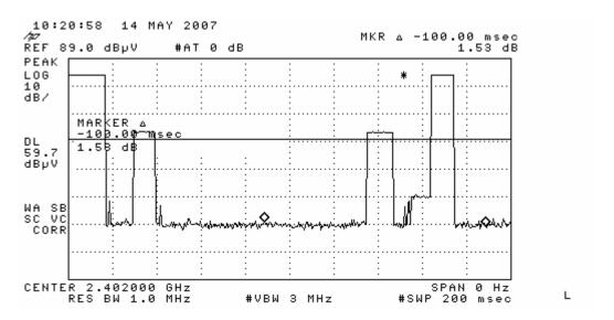
Graph below shows on time for the pulse during the 100ms window.
