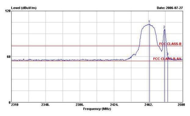
High Band Edge Plot on Configuration IEEE 802.11b / 2462 MHz and Bluetooth / 2480 MHz (AVG reading)
