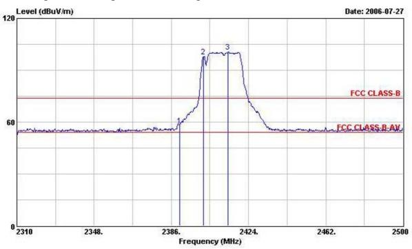
Low Band Edge Plot on Configuration IEEE 802.11g / 2412 MHz and Bluetooth / 2402 MHz (AVG reading)
