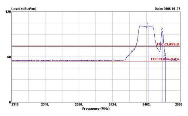
High Band Edge Plot on Configuration IEEE 802.11g / 2462 MHz and Bluetooth / 2480 MHz (AVG reading)
