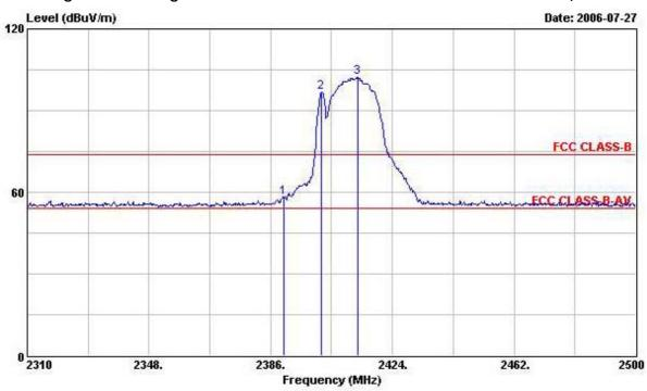
Low Band Edge Plot on Configuration IEEE 802.11b / 2412 MHz and Bluetooth / 2402 MHz (AVG reading)
