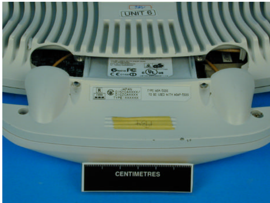
Photo 4: WSM5030 2.4GHz Integral Antenna Outside Case Rear Showing Connection to WSAP5030
