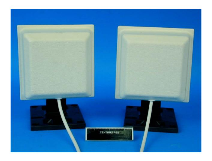
Photograph 5 Front View of 5GHz Patch Antennas
