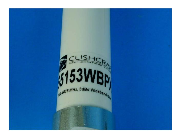
Photograph 11 View of 5GHz Omni Directional Antenna
