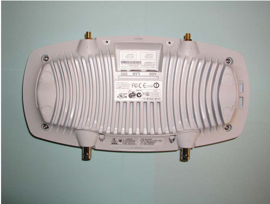
Photo 1; WSAP5030 External Antenna connections
