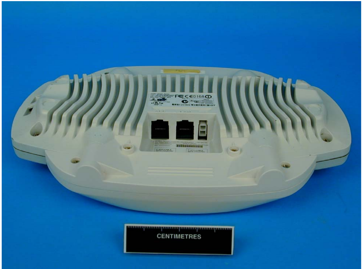
Photograph 4 Rear View Symbol WSAP 5030 Access Port with WSM 5030 RF Module and Integral Antennas (2.4GHz & 5.15-5.25GHz only)
