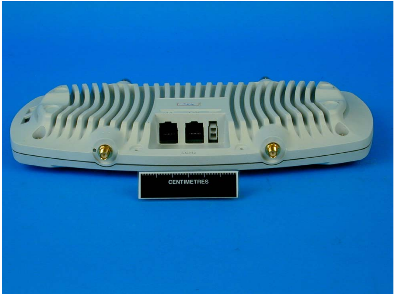
Photograph 6 Rear View Symbol WSAP 5030 Access Port with WSM 5030 RF Module and Antenna connectors (2.4GHz & 5.25-5.35 and 5.725-5.830GHz)
