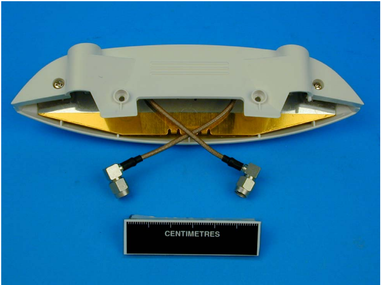
Photograph 9 Internal View Symbol WSAP 5030 Access Port Integral Antennas (5.15-5.25GHz only)
