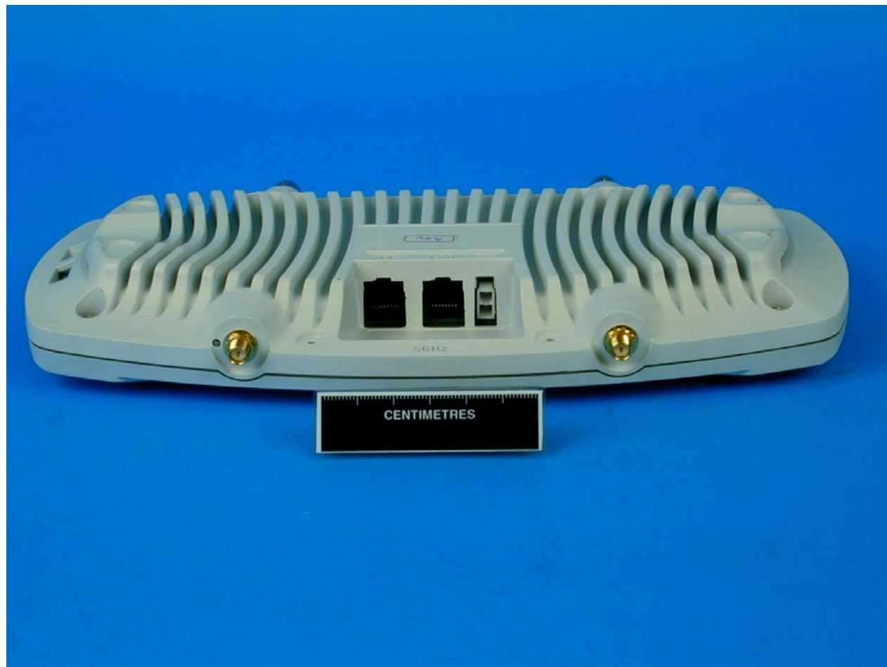
Photograph 6 Rear View Symbol WSAP 5030 Access Port External Antenna Connectors (5.25-5.35 and 5.725-5.825GHz)
