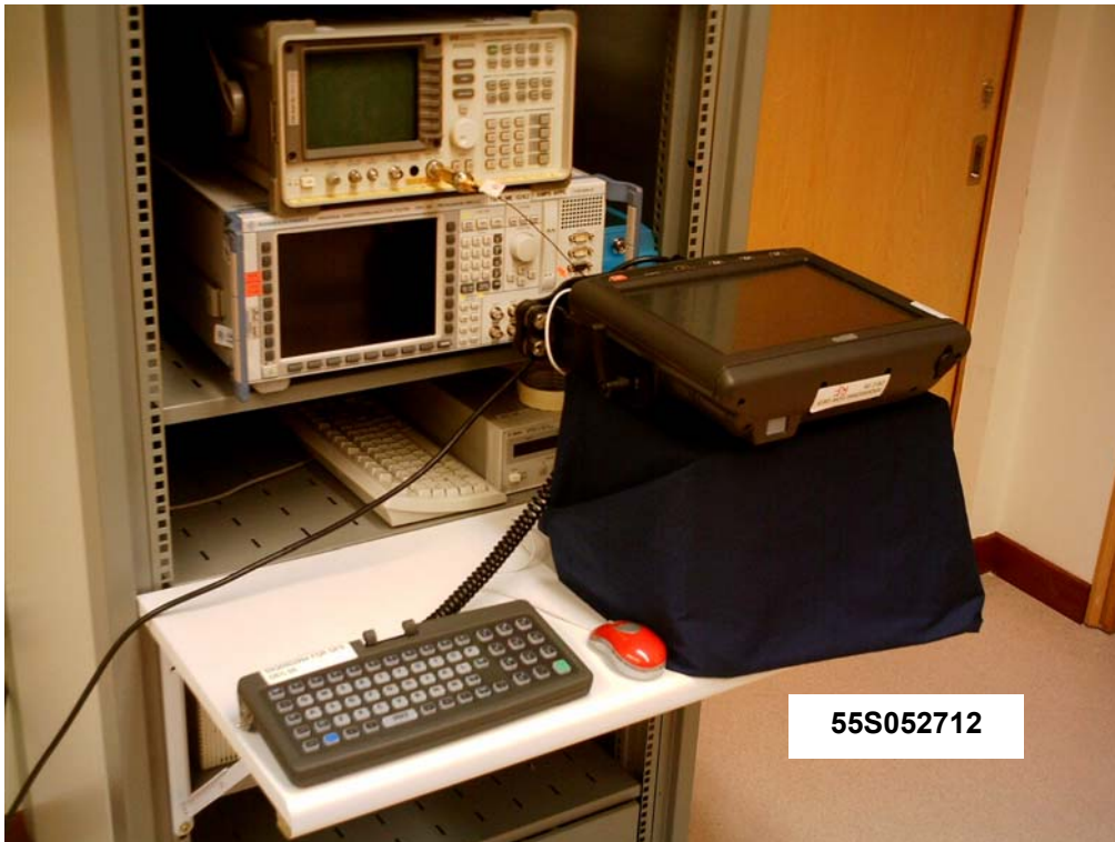
Carrier Frequency Separation Test Setup
