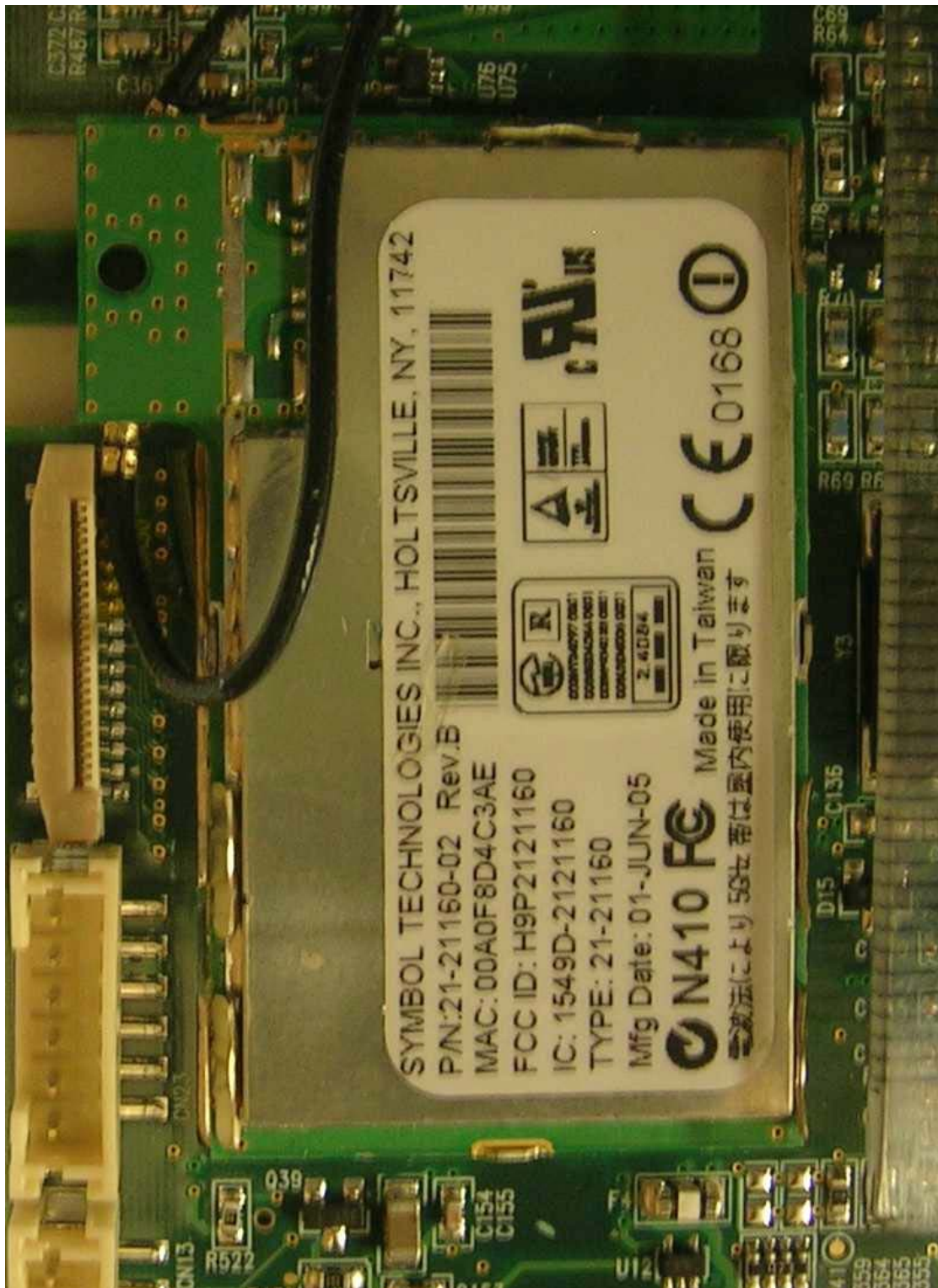
WLAN (802.11a/b/g) Module (With RF Shield)
