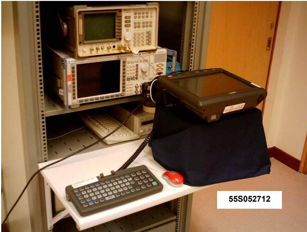
Spectrum Bandwidth (20dB Bandwidth Measurement) Test Setup
