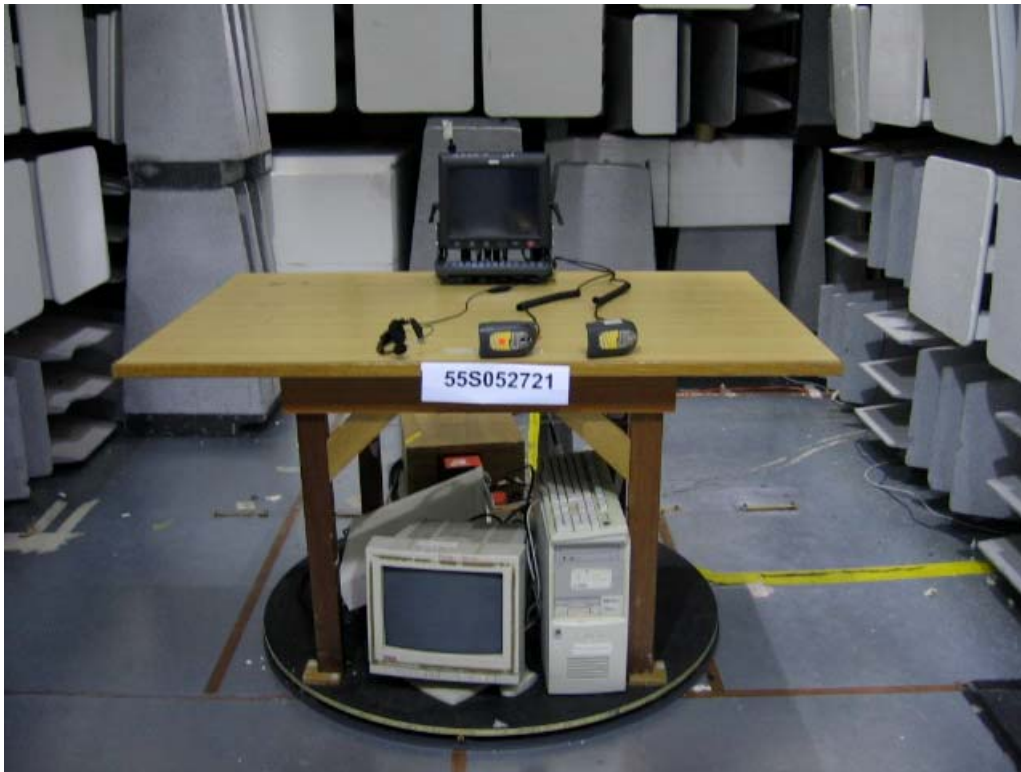
Maximum Peak Power Test Setup
