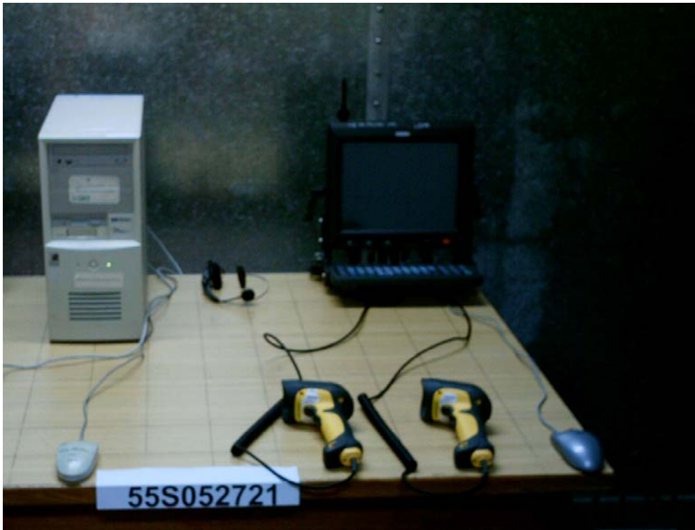
Conducted Emissions Test Setup (Front View)
