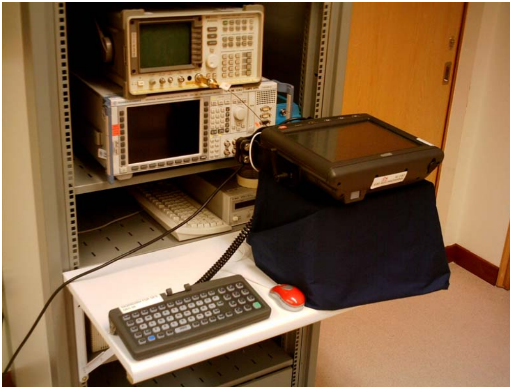
Maximum Output Power Test Setup
