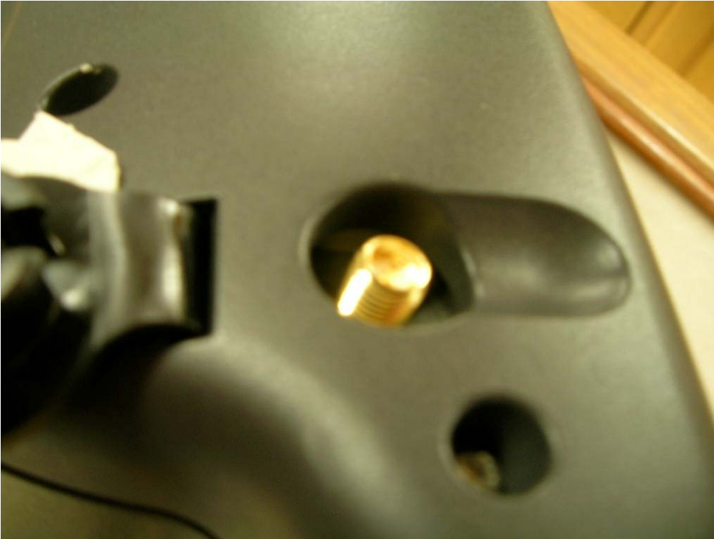
Antenna Port on the EUT
