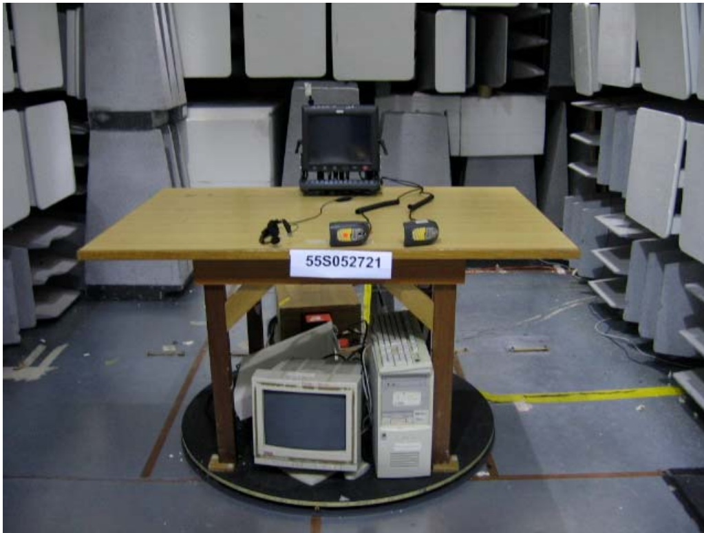
Maximum Peak Power Test Setup
