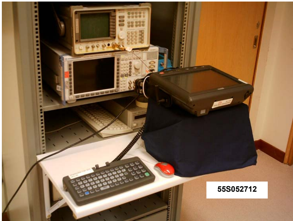
Average Frequency Dwell Time Test Setup
