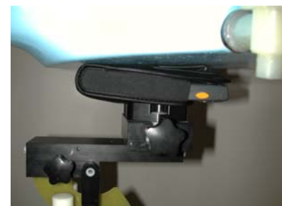
Figure 17. Body SAR Test Setup w/Holster
