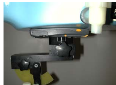
Figure 18. Hand SAR Test Setup
