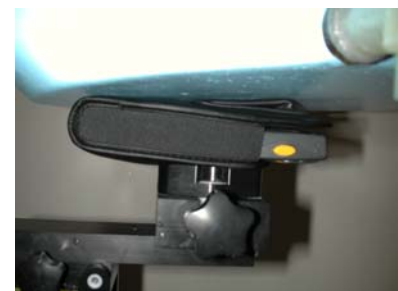
Figure 17. Body SAR Test Setup w/Holster
