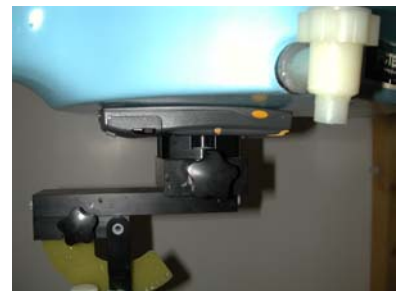
Figure 18. Hand SAR Test Setup
