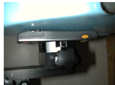
Figure 18. Hand SAR Test Setup
