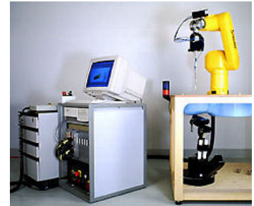
Fig. 1 SAR Test Setup
