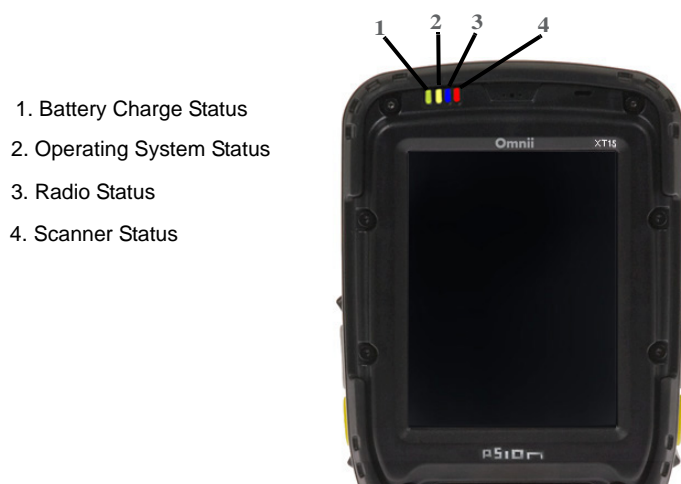
Figure 2-3 LED Status Indicators
