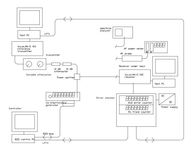
Figure 1, measurement test set-up.
