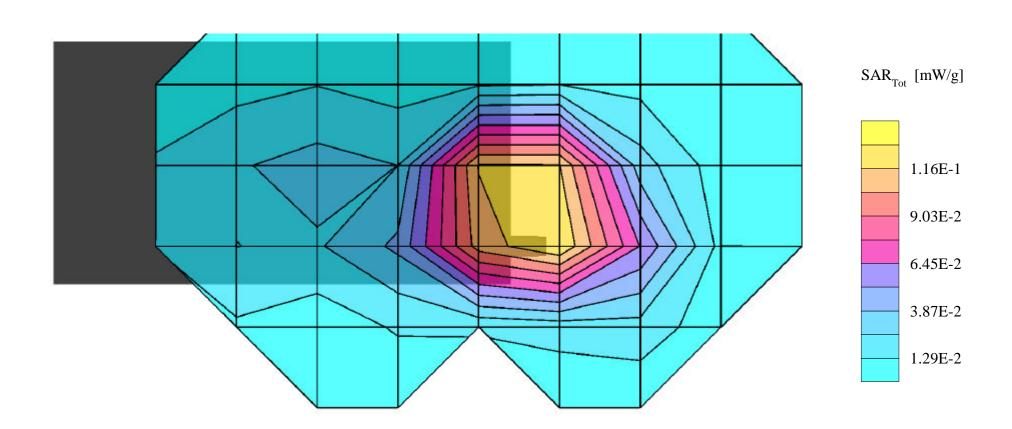
SAM~Phantom;~Flat~Section;~Probe:ET3DV6-SN1677;~ConvF(4.90,4.90,4.90) Med. Parameters 1900 MHz Muscle:  $\sigma=1.55~mho/m~\epsilon_r=54.9~\rho=1.00~g/cm^3;~Antenna~Position$  -- In; Crest Factor 8.0 SAR (1g): 0.156 ~mW/g,~SAR~(10g): 0.0999 ~mW/g
