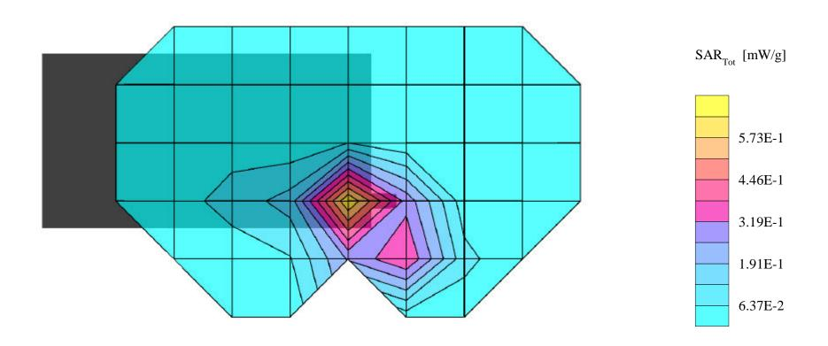
SAM~Phantom;~Flat~Section;~Probe:ET3DV6-SN1677;~ConvF(4.90,4.90,4.90) Med. Parameters 1900 MHz Muscle:  $\sigma=1.55~mho/m~\epsilon_r=54.9~\rho=1.00~g/cm^3;~Antenna~Position$  -- In; Crest Factor 8.0 SAR (1g): 0.165 ~mW/g,~SAR~(10g): 0.106 ~mW/g
