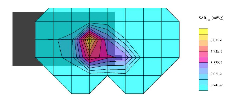
SAM~Phantom;~Flat~Section;~Probe:ET3DV6-SN1677;~ConvF(4.90,4.90,4.90) Med. Parameters 1900 MHz Muscle:  $\sigma=1.55~mho/m~\epsilon_r=54.9~\rho=1.00~g/cm^3;~Antenna~Position$  -- In; Crest Factor 8.0 SAR (1g): 0.897 ~mW/g,~SAR~(10g): 0.532 ~mW/g
