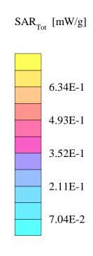
SAM~Phantom;~Flat~Section;~Probe:ET3DV6-SN1677;~ConvF(4.90,4.90,4.90) Med. Parameters 1900 MHz Muscle:  $\sigma=1.55~mho/m~\epsilon_r=54.9~\rho=1.00~g/cm^3;~Antenna~Position$  -- In; Crest Factor 8.0 SAR (1g): 0.631 ~mW/g,~SAR~(10g): 0.377 ~mW/g
