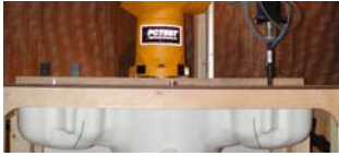
Figure 5.1 SAM Twin Phantom
