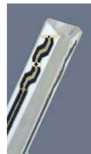
Figure 3.2 Probe Thick-Film Technique
