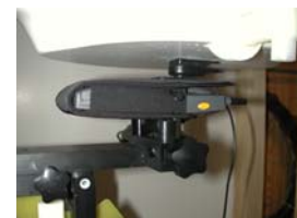
Figure 14.1 Body SAR Test Setup -- Fixed Position --
