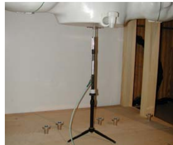
Figure 12.1 Dipole Validation Test Setup
