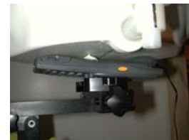
Figure 14.1 Body SAR Test Setup -- Back Side --
