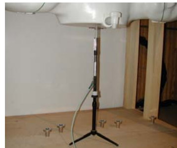
Figure 12.1 Dipole Validation Test Setup
