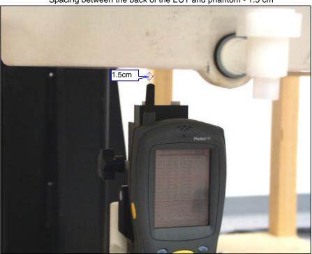
EUT Set-up Configuration 4 Spacing between the back of the EUT and phantom - 1.5 cm
