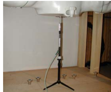
Figure 12.1 Dipole Validation Test Setup
