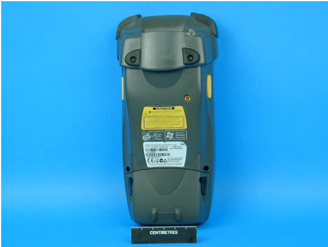
Figure 38. Rear view of the Symbol Portable Data Terminal, PDT8056. NOTE: Shown with optional strap attached – not attached for SAR Assessment.
