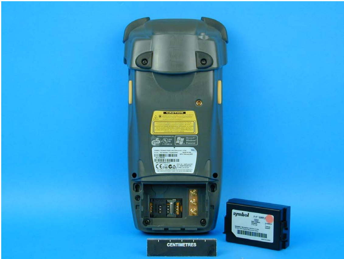
Figure 39. Rear View of the Symbol Portable Data Terminal, PDT8056, with the battery removed.
