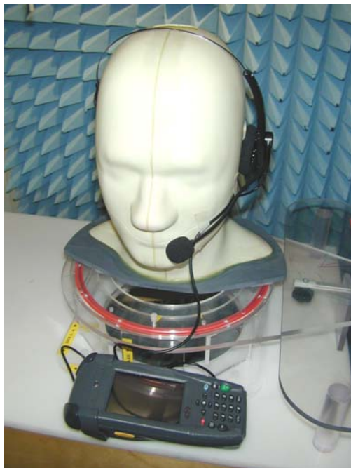
Figure 36. Positional photograph of Symbol Headset in the LH CheekTouch Position Connected to the PDT8056 against the SAM Phantom.
