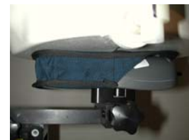
Figure 14.1 Body SAR Test Setup -- w/ Holster --
