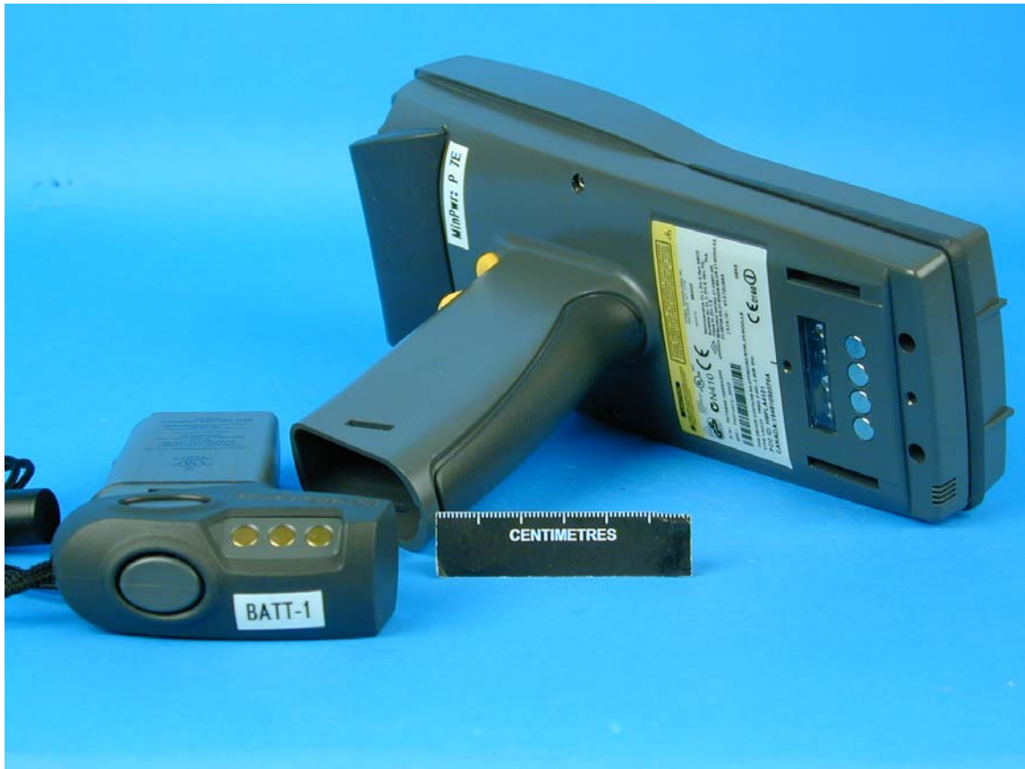
Figure 39. Rear View of the Symbol Portable Data Terminal, PDT687C, with the battery removed.
