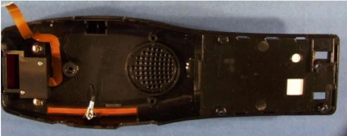
Antenna installed in DP4046 Voice communication device
