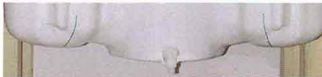
Figure 7.2 SAM Twin Phantom shell
