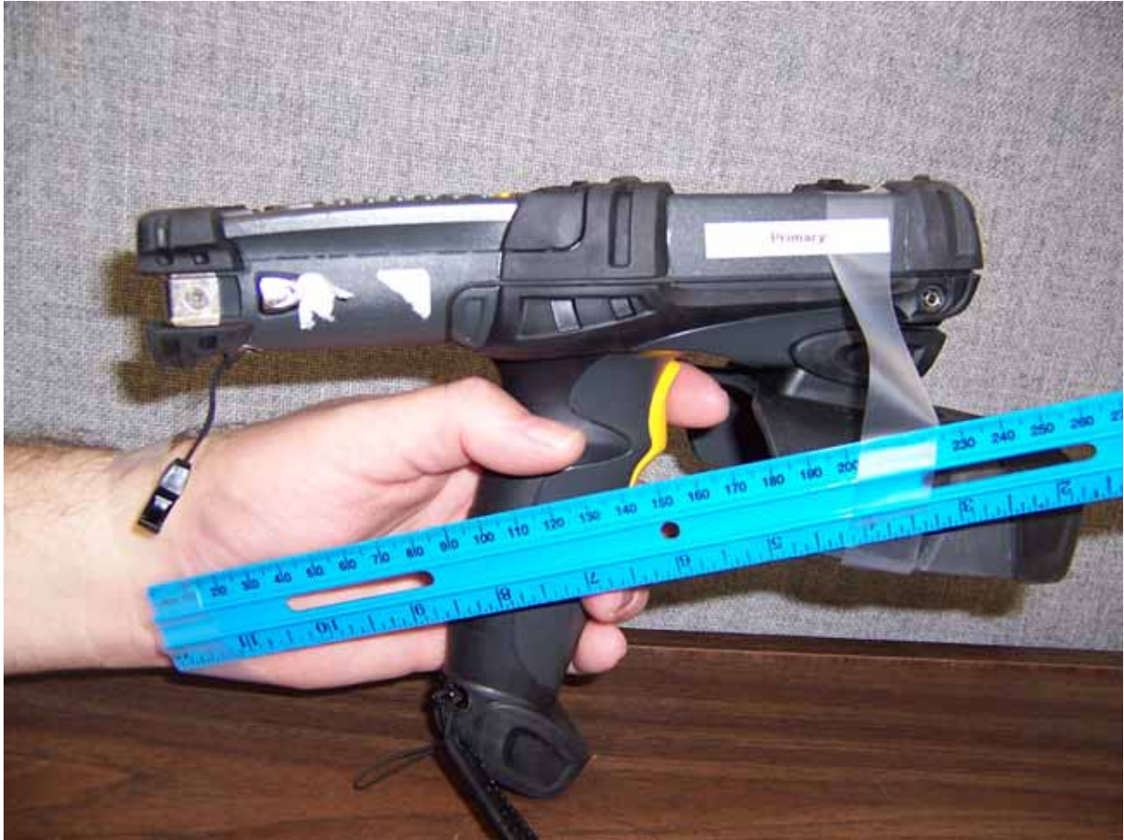
Figure 1. Separation Distance to Antenna
