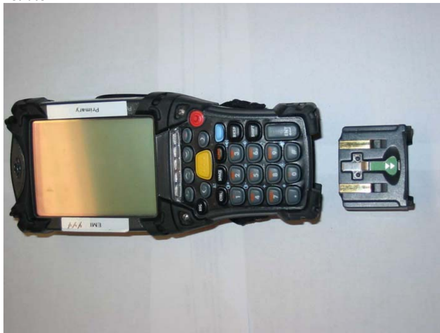
Figure 4 – MC9063 with Battery Removed
