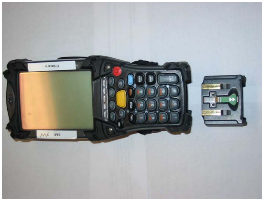
Figure 4 – MC9063 with Battery Removed
